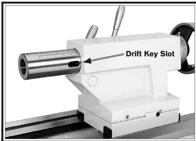
Figure 53. Drift key slot in the side of the quill.
